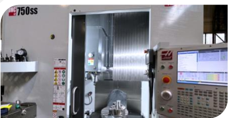
5-axis Haas UMC 750 SS XYZBC 762 x 508 x 508 mm, SK40, CTS
