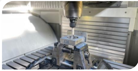
5-axis DMG DMU 60 T XYZ 630 x 560 x 560 mm, SK40, CTS
