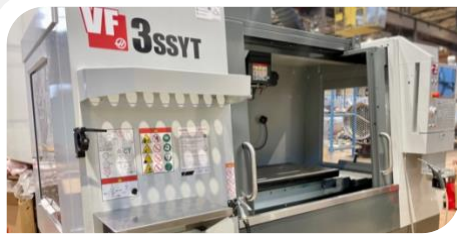
3-axis Haas VF3 SSYT XYZ 1016 x 660 x 635 mm, SK40, CTS
