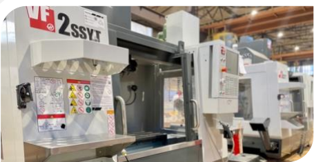
3-axis Haas VF2 SSYT XYZ 762 x 508 x 508 mm, SK40, CTS
