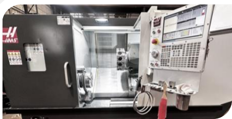
Haas ST 30 Y Turn-Mill XYZ 239 x 101 x 826 mm, 3400 rpm, 22.4 kW
