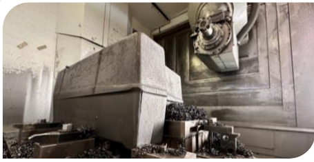
5-axis DMG DMU 125P Hi Dyn, 3 pcs. XYZ 1250 x 880 x 800 mm, SK50, CTS
